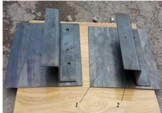
Fig. 4. – Prototype frame: 1 – sheathing sheet; 2 – Z-shaped profile
